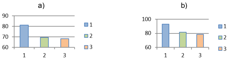
Figure 1. Diagram of comparison of compressive forces values depending on the type of nodal joints: a) rigid joint, b) hinged joint. (1-elastic solution, 2-solution by 1 st limit state, 3-solution by 2 nd limit state)
