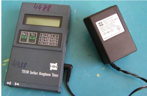
Figure 5.5 - Electronic TR100 Surface Roughness Tester for Roughness Measurement
