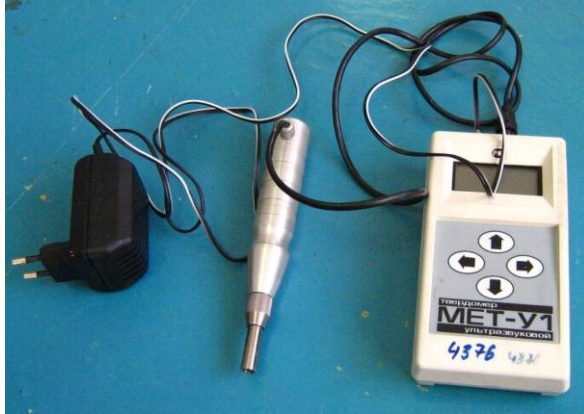
Figure 5.3 - MET-U1 device for measuring hardness by the Vickers's method
