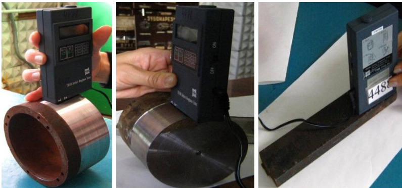
Figure 5.6 - Measurement of roughness of the processed samples
