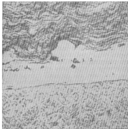
Figure 3.4 - Spray Coating Structure
