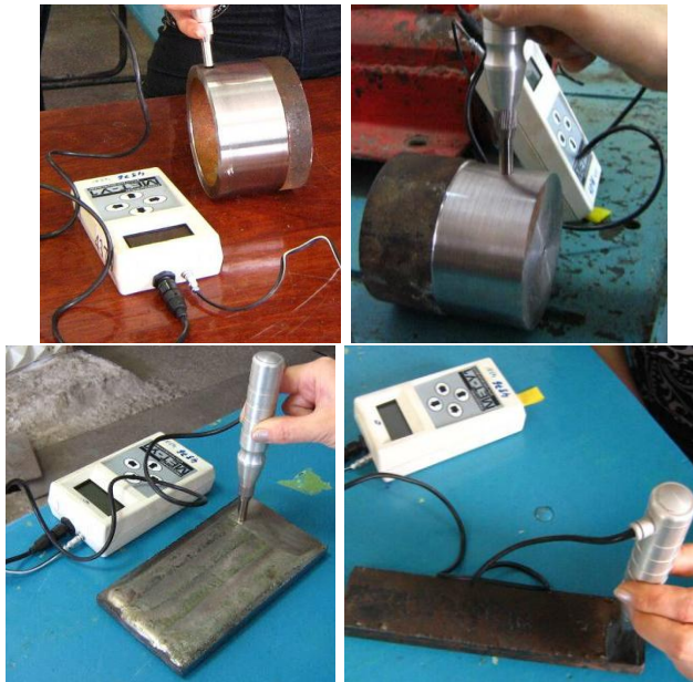
Figure 5.4 - Hardness Measurements of Processed Samples
