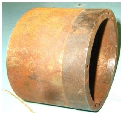
Figure 5.11 - Cylindrical sample of 35L steel for research
