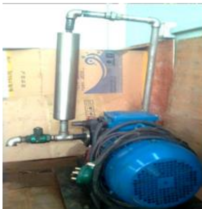
Figure 8. Appearance of the assembled cavitator
