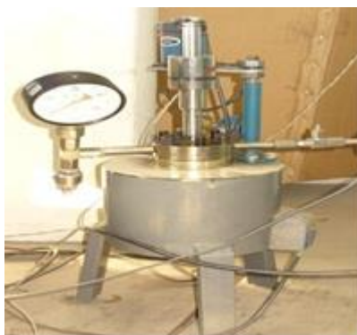
Figure 10. High Pressure Reactor
