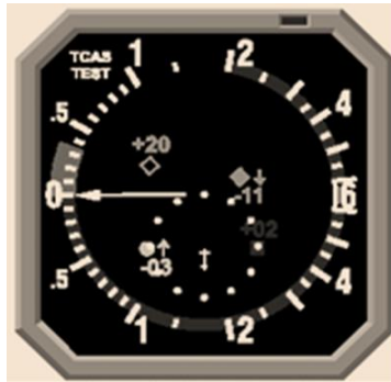
Figure 4.7 – Image of the test picture on the display of the VSI / TRA indicator
