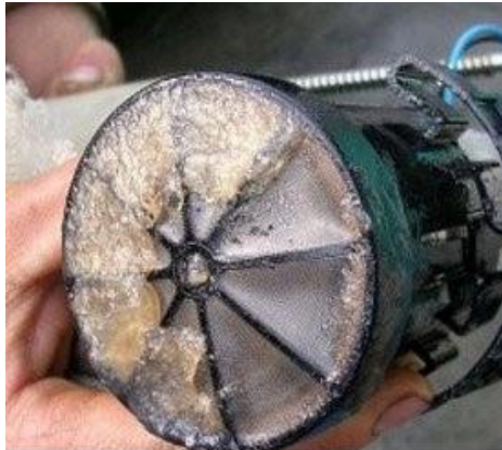
Figure 2. Defective fuel pump
