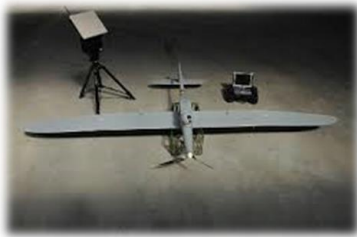
Fly Eye "WB Electronics" tactical radius up to 50 km
