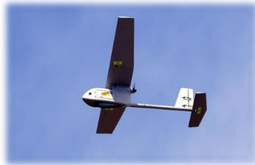
RQ-11B Raven "AeroVironment" tactical radius up to 10 km
