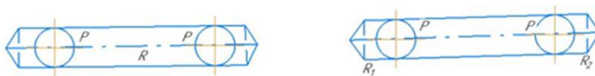
Figure 3.20. Scheme of interaction of the support base with soil rocks at two-point contact
