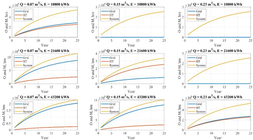
Figure 2.21 – Operating costs of the power supply system with the mini-PSPP (two hydroturbines on the 500m level) during the operation period for different values of hydroturbine water consumption and average daily power consumption with power costs  $\alpha_{ee} = 140.07 \text{ UAH}/\text{MWh}$
