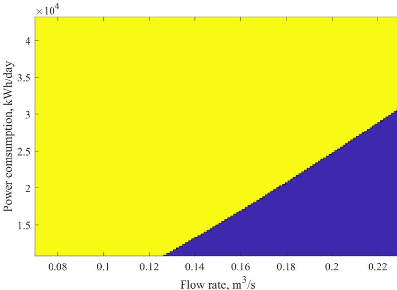
Figure 2.16 – Power supply system of the 500m level with a single turbine introduced, which is efficient in terms of the NPV depending on changes in load and water consumption with the tariff  $\alpha_{ee} = 140.07 \text{ UAH}/MWh$
