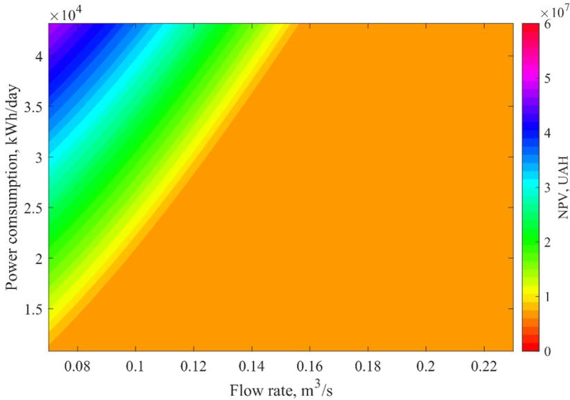
Figure 2.31 – Dependence  $NPV = f(Q, E)$  for power system two hydroturbines introduced on the 500m level and two hydroturbines introduced on the 940m level with the tariff of  $\alpha_{ee} = 140.07 \text{ UAH/MWh}$
