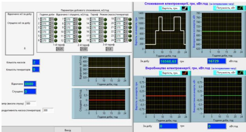
Figure 2.3 – Power consumption during the day at the iron ore underground mine
