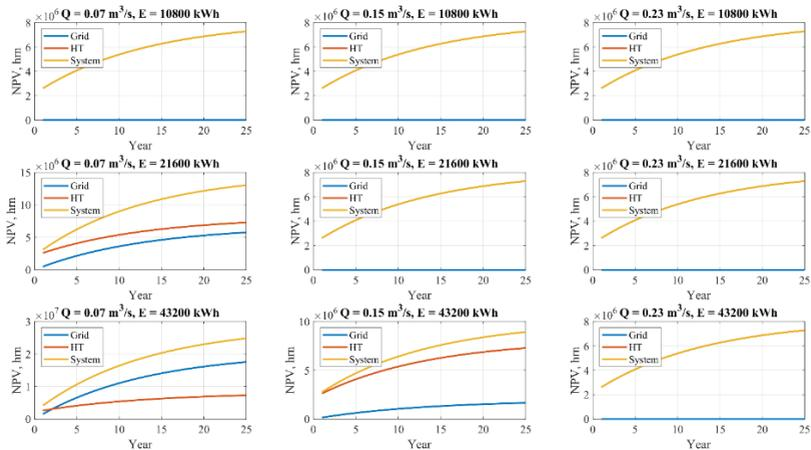
Figure 2.30 – NPV of the power supply system with the mini-PSPP (two and two hydroturbines on the 500m and 940m levels) during the operation period for different values of hydroturbine water consumption and average daily power consumption with power costs of
