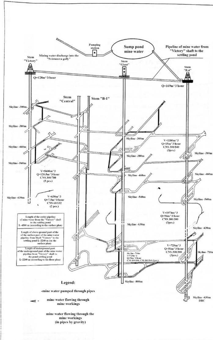
Figure 1.14 – Water pumping by water drainage facilities of the abandoned Hihant-Hlyboka underground mine (Kryvyi Rih)
