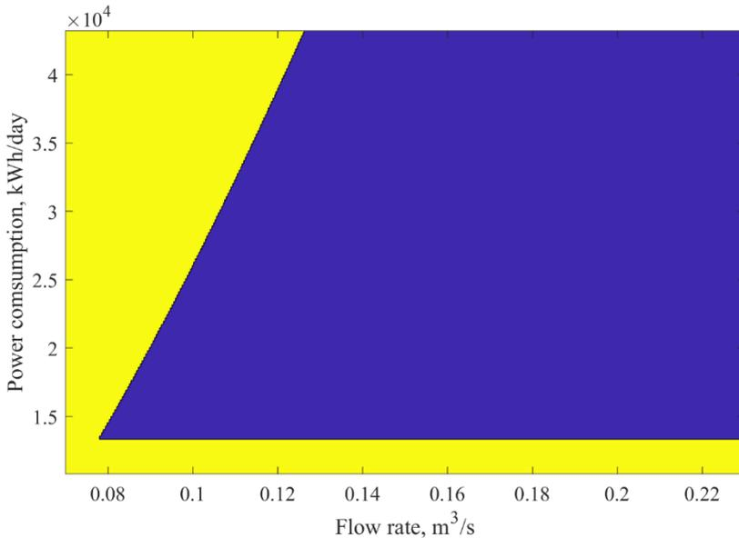
Figure 2.32 – Power system with four hydroturbines introduced on the 500m and 940m levels which is efficient in terms of the NPV depending on changes in load and water consumption with the tariff of  $\alpha_{ee} = 140.07 \text{ UAH}/\text{MWh}$
