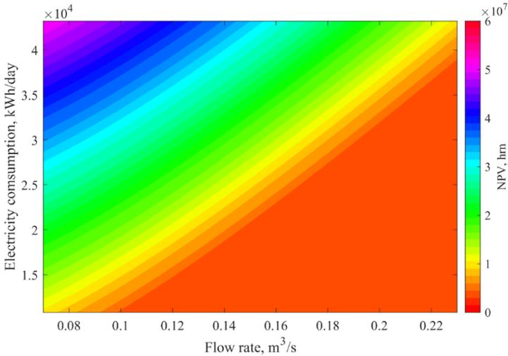
Figure 2.23 – Dependence  $NPV = f(Q, E)$  for two hydroturbines introduced on the 500m level with the tariff  $\alpha_{ee} = 140.07 \text{ UAH}/\text{MWh}$
