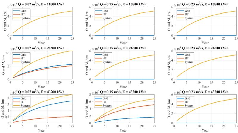
Figure 2.29 – Operating costs of the power supply system with the mini-PSPP (two and two hydroturbines on the 500m and 940m levels) during the operation period for different values of hydroturbine water consumption and average daily power consumption with power costs
