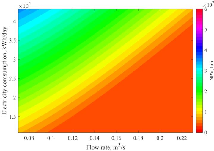
Fig. 2.19. Dependence  $NPV = f(Q, E)$  for two hydroturbines introduced on the 500m level ( $\alpha_{ee} = 93.38 \text{ UAH/MWh}$ )
