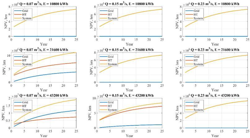
Figure 2.26 – NPV of the power supply system with the mini-PSPP (two and two hydroturbines on the 500m and 940m levels) during the operation period for different values of hydrogenerator water consumption and average daily power consumption with power costs  $\alpha_{ee} = 93,38 \text{ UAH}/\text{MWh}$
