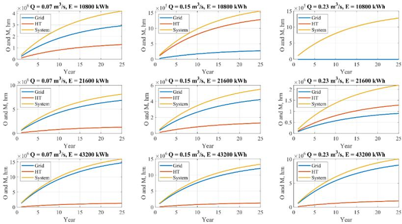
Figure 2.9 – Operating costs of the power supply system with the mini-PSPP for different values of hydroturbine water consumption and average daily power consumption with the power cost of  $\alpha_{ee} = 93,38 \text{ UAH}/\text{MWh}$
