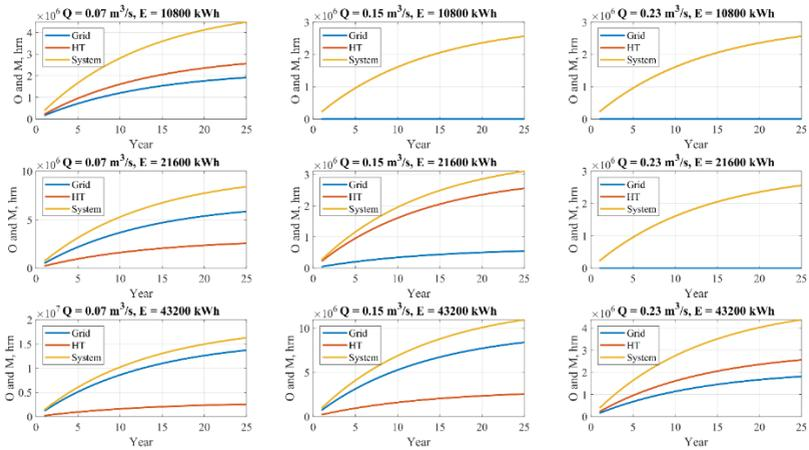
Figure 2.17 – Operating costs of the power supply system with the mini-PSPP (two hydroturbines on the 500m level) during the period of operation for different values of hydroturbine water consumption and average daily power consumption with power costs  $\alpha_{ee} = 93.38 \text{ UAH}/\text{MWh}$
