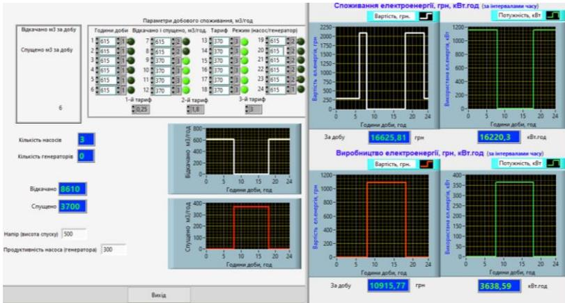
Figure 2.5 – Power consumption and generation of a balanced system at the iron ore underground mine
