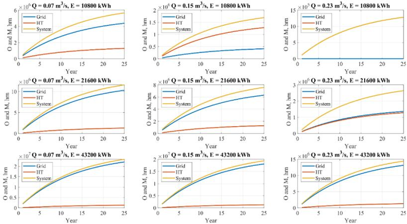
Figure 2.13 – Operating costs of the power supply system with mini-PSPPs during the operation period for different values of hydroturbine water consumption and average daily power consumption with the power cost  $\alpha_{ee} = 140.07 \text{ UAH/MWh}$
