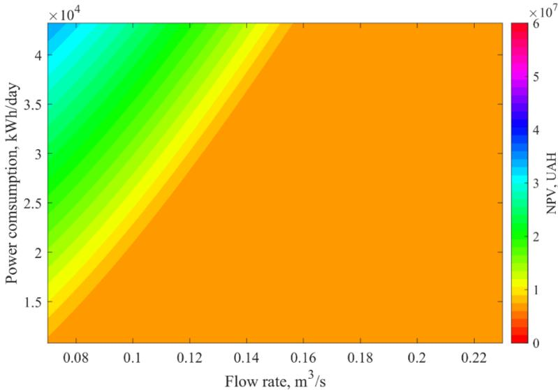
Figure 2.27 – Dependence of the NPV of the combined power supply system on hydroturbine water consumption and the level of power consumption  $NPV = f(Q, E)$  with two hydroturbines introduced on the 500m level and two hydroturbines introduced on the 940m level with the tariff of  $\alpha_{ee} = 93,38$  UAH/MWh
