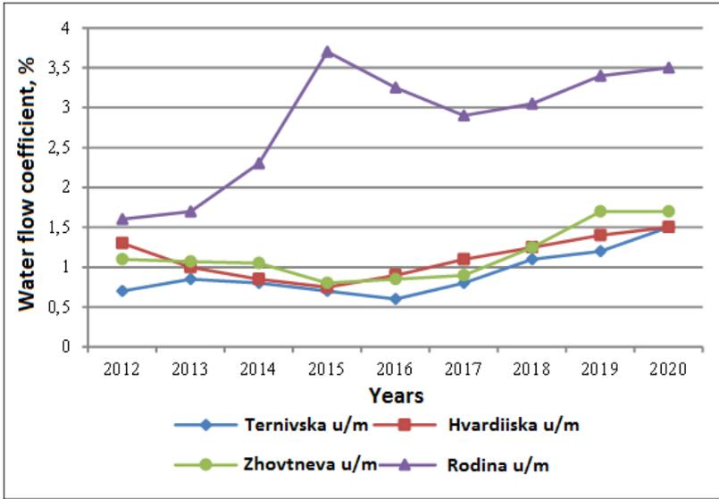
Figure 1.16 – Water flow coefficient of some iron ore underground mines of Kryvyi Rih iron ore basin
