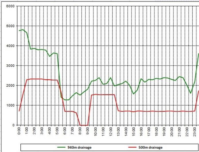
Figure 1.17 – Curves of active power consumption by electric drives of mine water drainage facilities of Rodina underground mine (Kryvyi Rih)
