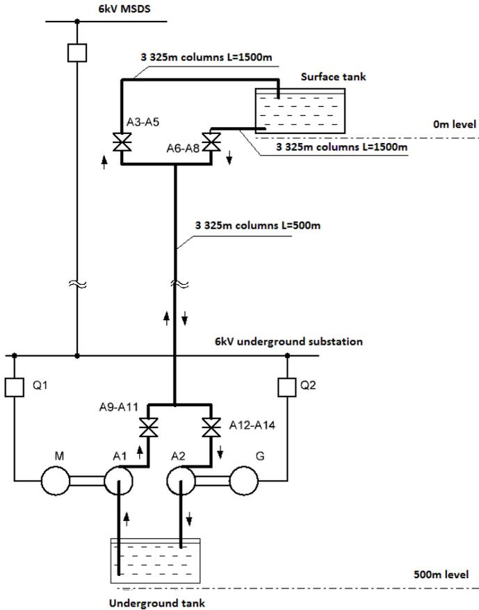
Fig. 2.7 – Peak PSPP with a common pressure pump column at the iron ore underground mine
