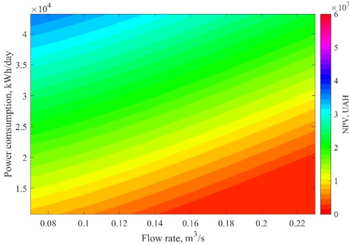
Figure 2.11 – Dependence of the NPV of the combined power supply system on hydrogenerator water consumption and the level of power consumption with a single hydrogenerator introduced on the 500m level with the tariff  $\alpha_{ee} = 93,38 \text{ UAH}/\text{MWh}$
