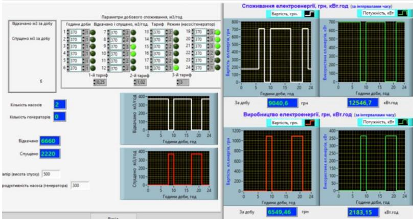
Figure 2.4 – Curves of power consumption and generation during the day at the iron ore underground mine
