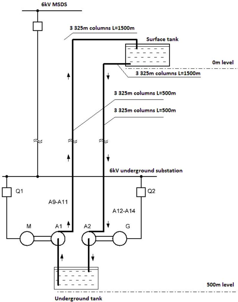
Figure 2.8 – Peak PSPP with separate pressure pump columns of an iron ore underground mine
