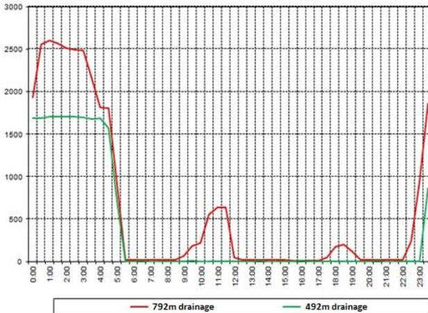
Figure 1.17 – Curves of active power consumption by electric drives of mine water drainage facilities of Hvardiiska underground mine (Kryvyi Rih)
