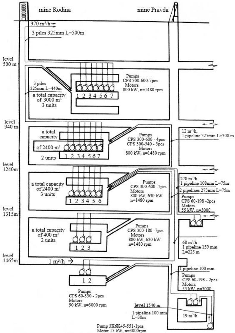
Figure 1.13 – Water pumping by water drainage facilities of the integrated water drainage complex of Rodina and Pravda underground mines (Kryvyi Rih)
