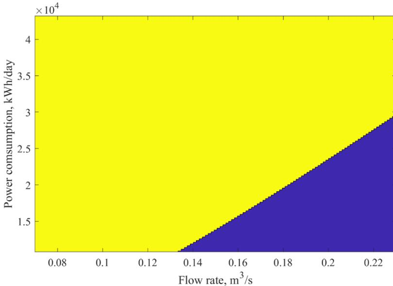
Figure 2.12 – Power supply system of the 500m level with a single turbine introduced which is efficient in terms of the NPV depending on changes in load and water consumption with the tariff  $\alpha_{ee} = 93.38 \text{ UAH}/\text{MWh}$
