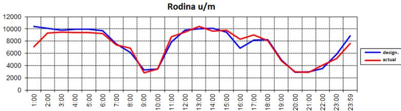
Figure 1.2 – Designed and actual consumption of active power at some iron ore underground mines of Ukraine (September 25, 2020)
