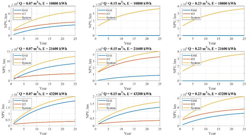
Figure 2.22 – NPV of the power supply system with the mini-PSPP (two hydroturbines on the 500m level) during the operation period for different values of hydroturbine water consumption and average daily power consumption with power costs  $\alpha_{ee} = 140.07 \text{ UAH}/\text{MWh}$
