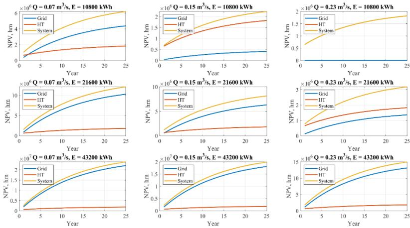
Figure 2.14 – NPV of the power supply system with mini-PSPPs during the operation period for different values of hydroturbine water consumption and average daily power consumption with the power cost  $\alpha_{ee} = 140.07 \text{ UAH/MWh}$
