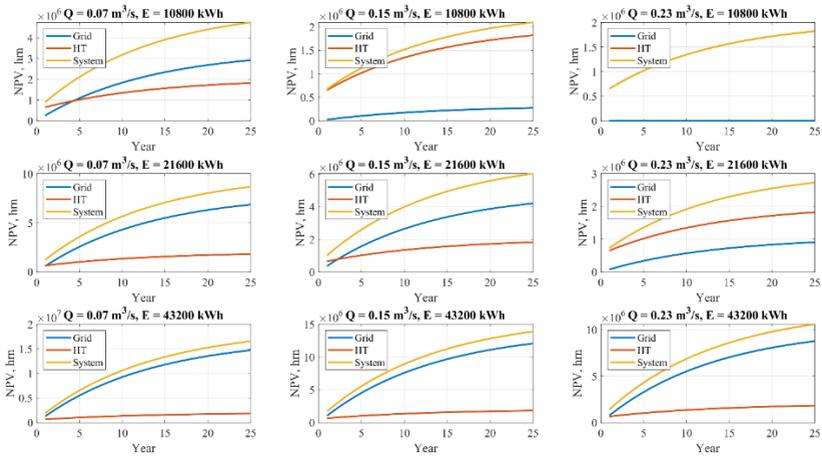
Figure 2.10 – NPV of the power supply system with the mini-PSPP for different values of hydroturbine water consumption and average daily power consumption with the power cost of  $\alpha_{ee} = 93,38 \text{UAH}/\text{MWh}$
