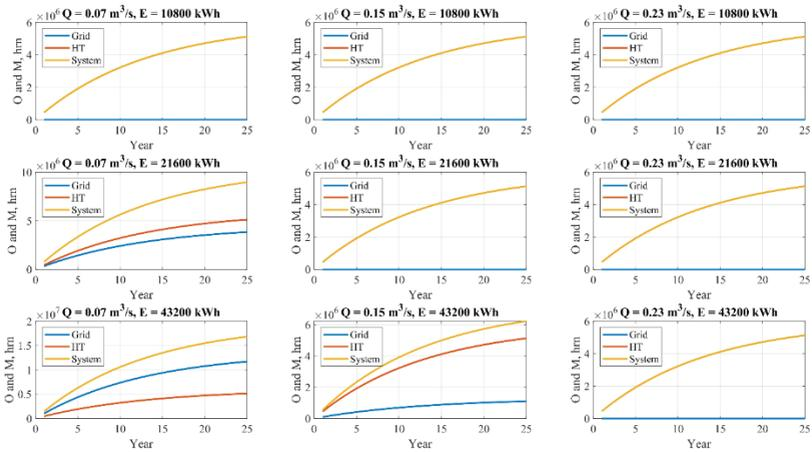
Figure 2.25 – Operating costs of the power supply system with the mini-PSPP (two and two hydroturbines) on the 500m and 940m levels) during the operation period for different values of hydroturbine water consumption and average daily power consumption with power costs of
