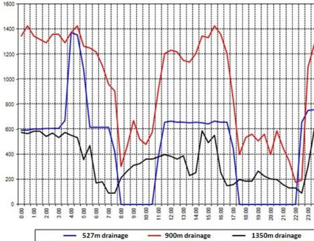
Figure 1.17 – Curves of active power consumption by electric drives of mine water drainage facilities of Ternivska underground mine (Kryvyi Rih)
