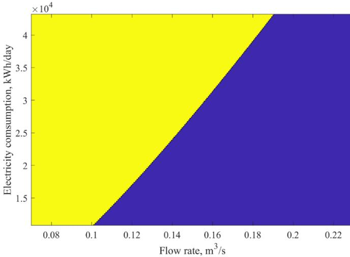
Figure 2.20 – Power supply system with two hydroturbines introduced on the 500m level which is efficient in terms of the NPV depending on changes in load and water consumption with the tariff of  $\alpha_{ee} = 93.38 \text{ UAH/MWh}$
