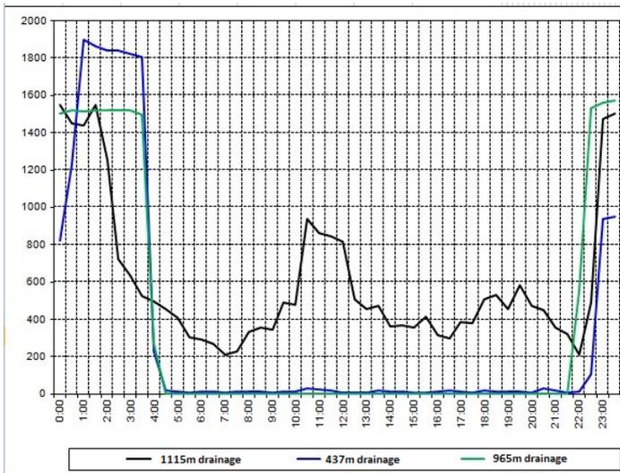
Figure 1.17 – Curves of active power consumption by electric drives of mine water drainage facilities of Oktiabrskaya underground mine (Kryvyi Rih)
