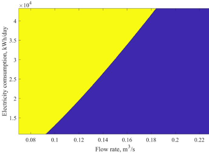
Figure 2.24 – Power system with two hydroturbines introduced on the 500m level which is efficient in terms of the NPV depending on changes in load and water consumption with the tariff  $\alpha_{ee} = 140.07 \text{ UAH}/\text{MWh}$
