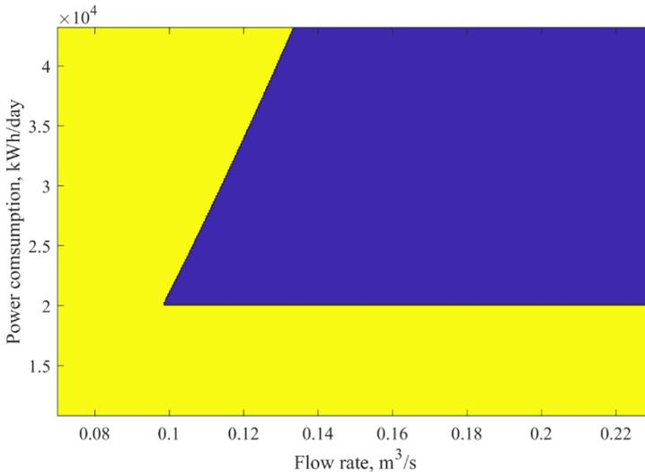
Figure 2.28 – Power supply system with four hydroturbines introduced on the 500m and 940m levels which is efficient in terms of the NPV depending on changes in load and water consumption with the tariff of  $\alpha_{ee} = 93,38 \text{ UAH/MWh}$
