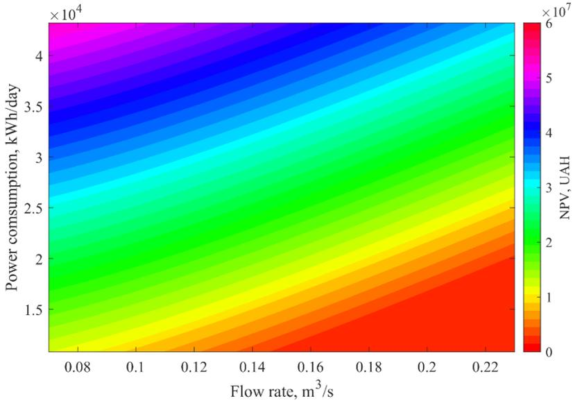
Figure 2.15 – Dependence of the NPV of the combined power supply system on hydroturbine water consumption and power consumption  $NPV = f(Q, E)$  with a single hydroturbine introduced on the 500m level with the tariff  $\alpha_{ee} = 140.07 \text{ UAH}/MWh$
