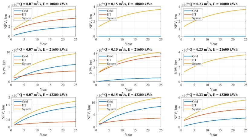
Figure 2.18 – NPV of the power supply system with the mini-PSPP (two hydroturbines on the 500m level) during the operation period for different values of hydroturbine water consumption and average daily power consumption with power costs  $\alpha_{ee} = 93.38 \text{ UAH}/\text{MWh}$
