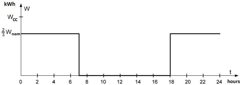
Figure 2.6 – Ideal curve of functioning of the synergistic water drainage facility and PSPPs:  $W_{cc}$  is volumes of centralized power consumption from the generating company;  $2/3 \cdot W_{nom}$  is the maximum allowable level of power consumption according to the ordered volumes of the enterprise for the current day
