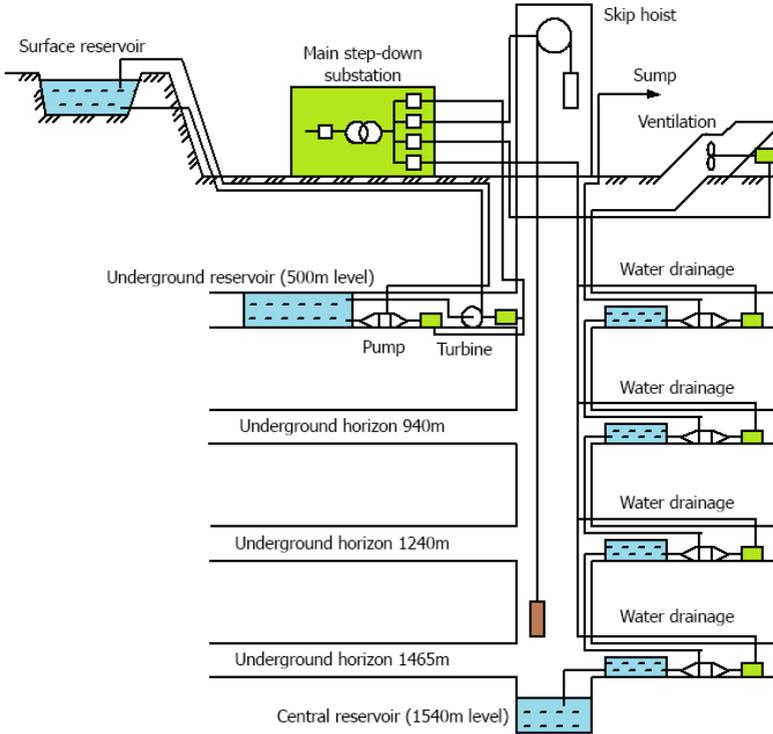
Figure 2.1 – Mine peak pump-storage power plant
